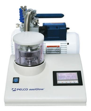
The PELCO easiGlow™ Glow Discharge Cleaning System is a compact, quick and easy-to-use standalone system. It is primarily designed for hydrophilization of TEM carbon support films which have the tendency to be hydrophobic. A glow discharge treatment with air will make the carbon film surface negatively charged (hydrophilic) which allows aqueous solution to spread easily.
